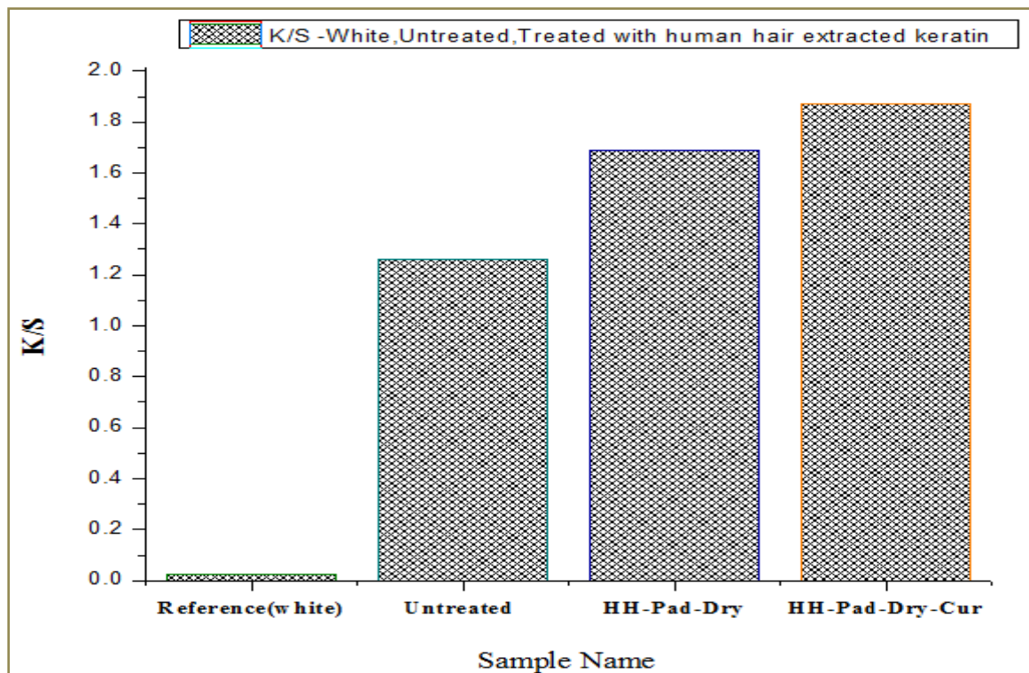
Figure 13: K/S value at \lambda_{max} (620 nm) for untreated and treated with human hair extracted keratin and dyed with DCT reactive blue dye
